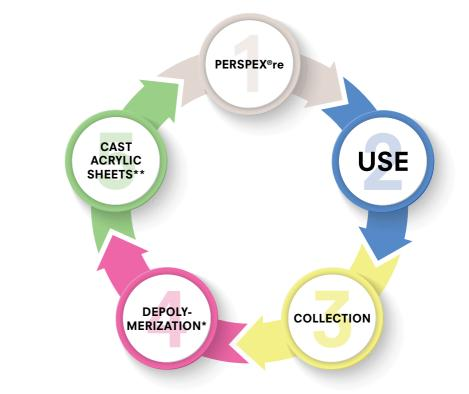
\* Depolymerization (Cracking and Distillation - production of rMMA, external waste management) \*\* Production of cast acrylic sheets (Polymerization)
