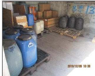
Photo of non-conformity No secondary containment nor safety label.JPG
